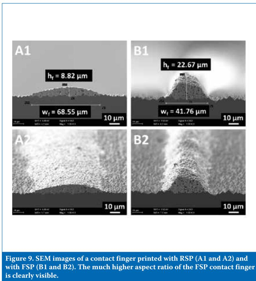
**Figure 9. SEM images of a contact finger printed with RSP (A1 and A2) and with FSP (B1 and B2). The much higher aspect ratio of the FSP contact finger is clearly visible.**
