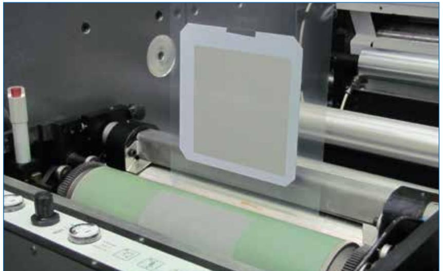
Figure 6. Transport of a Si wafer through the RSP printing unit by fixing it on a foil web.
