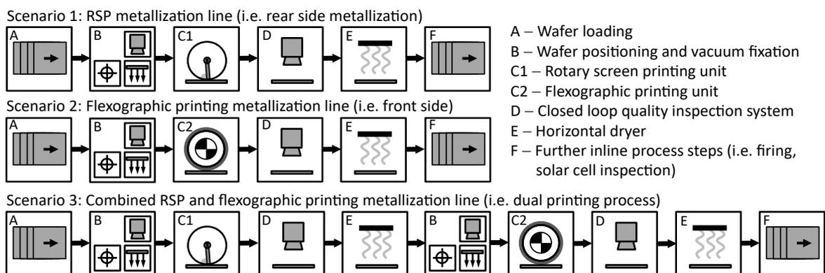
Figure 1. Illustrative presentation of different configurations for a back-end metallization line using rotary-printing methods. Scenarios 1 and 2 represent concepts for a rear-side metallization line using RSP and a front-side metallization line using FXP respectively. Scenario 3 combines both technologies in one metallization line (i.e. for a dual-printing process of busbars and contact fingers).
