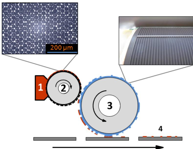
Figure 5. Schematic of a (theoretical) FXP unit for the metallization of silicon solar cells: from the ink reservoir (1), a defined amount of ink is transferred by the anilox roll (2) onto fine finger elements on the printing plate (3), and subsequently onto the silicon wafer (4).
