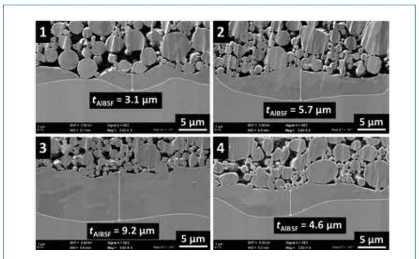
Figure 8. SEM cross-sectional images and local measurement of the resulting Al BSF depth after contact firing. Images 1 to 3 represent samples with RSP rear-side metallization and different cylinder screens. Image 4 is the reference sample with FSP rear-side metallization.
