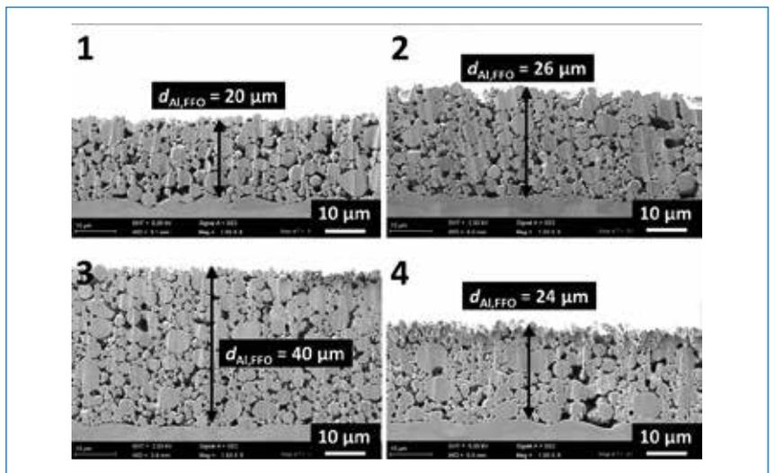
Figure 7. SEM cross-sectional images of the Al rear-side metallization after contact firing. Images 1 to 3 represent samples with RSP rear-side metallization and different cylinder screens. Image 4 is the reference sample with FSP rear-side metallization.
