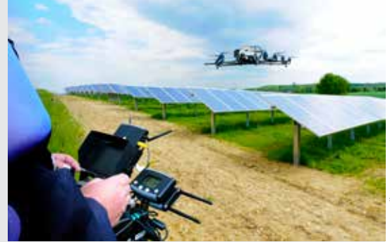
Drones can be used for visual and thermographic inspections of a plant during commissioning.
