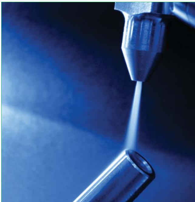
Figure 4. The CO 2 snow-jet does not use water and does not require manual handling.
