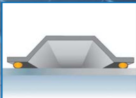
Bonding of back rails
