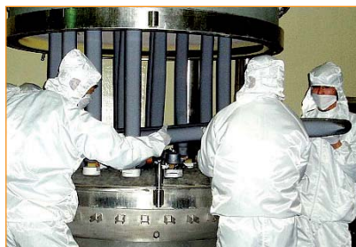
LDK Solar polysilicon rods produced by advanced Siemens process.
