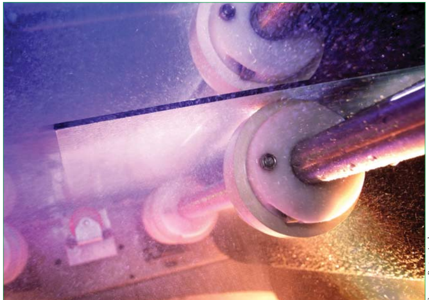
Figure 3. Glass washing is a common production step for all thin-film technologies.
