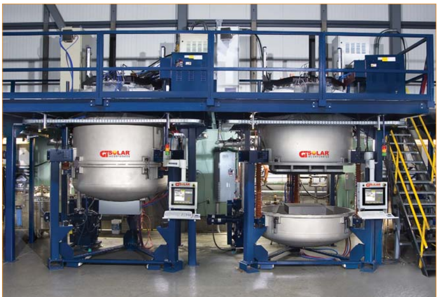
Figure 5. GT Solar's DSS450HP ingot growth furnace.
