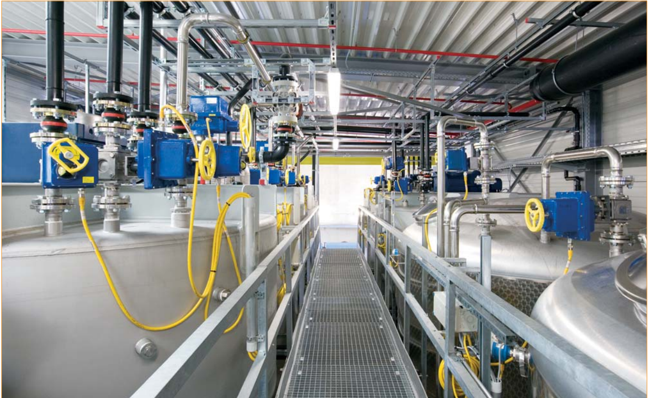
Figure 6. CRS Reprocessing Services' typical slurry recycling system.
