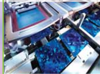
Precision Stencils and Screens, next-generation fine line deposition for increased cell efficiency
