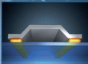
Bonding of back rails
