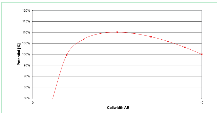
Figure 6. Schematic drawing showing the optimum width of a cell in a thin-film module.
