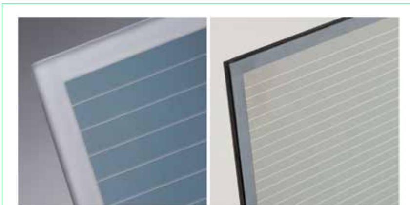
Figure 7. Picture of a CX1 module (left-hand picture) in comparison to a CX3 module (right-hand side) featuring optimized cell widths and improved package design. Details discussed in the text.
