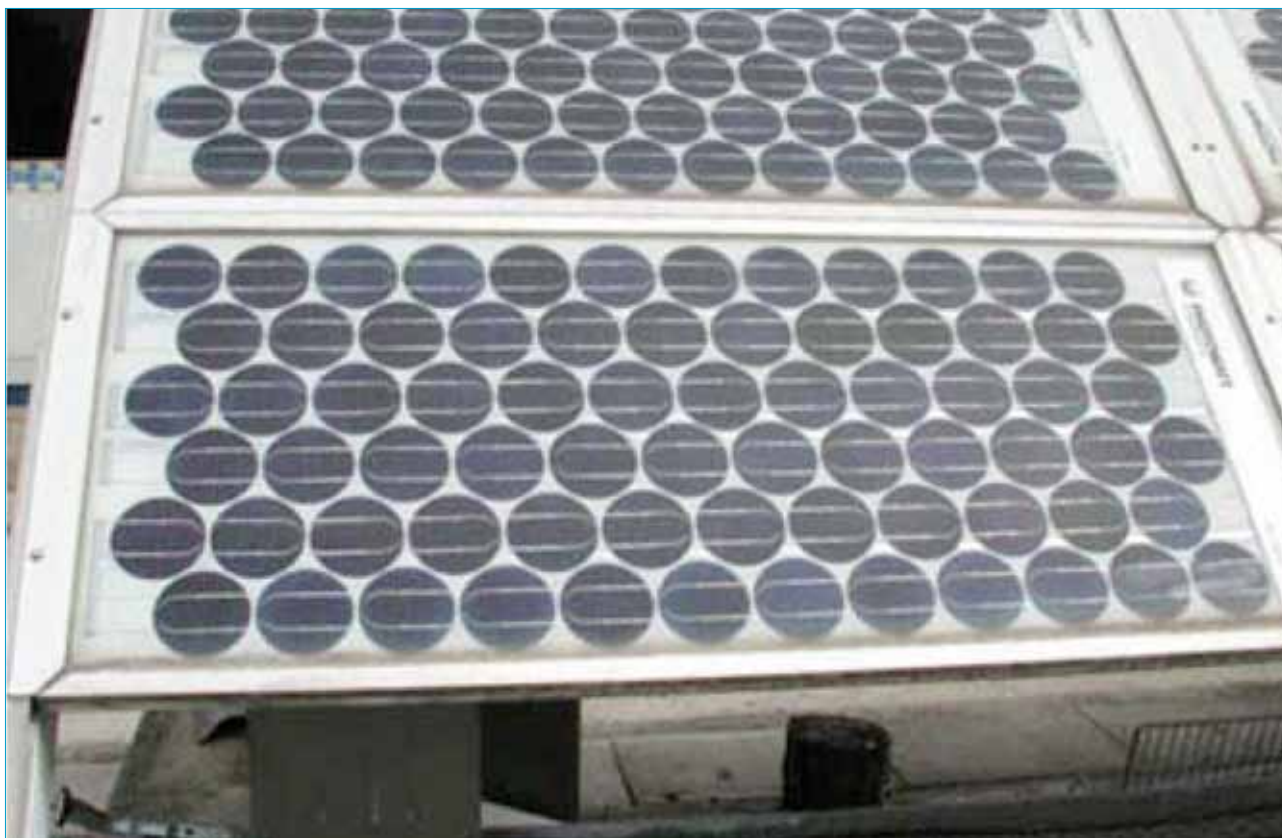
Figure 9. Monocrystalline silicon PV panel after 20 years of outdoor exposure.
