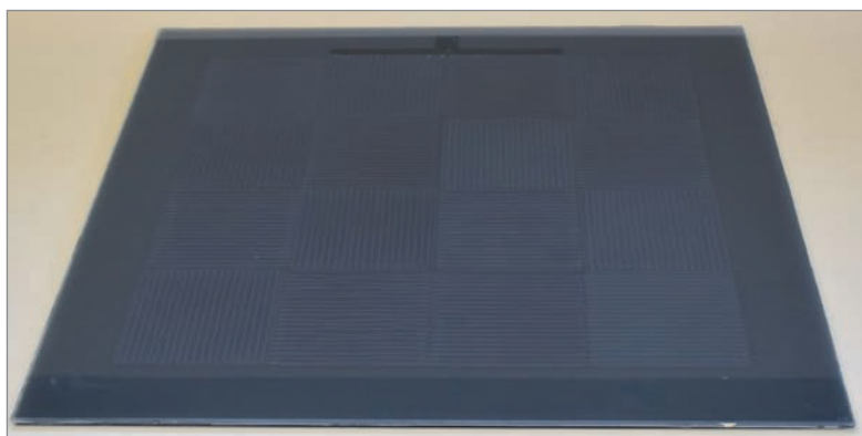
Figure 8. Example of a 4x4-cell module incorporating imec multi-wire interconnection technology.
