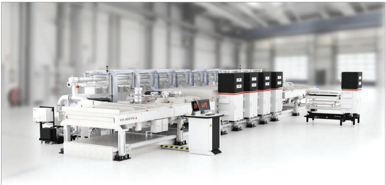
Figure 7. Example of TCO mass-production equipment: VON ARDENNE's XEA|nova L.
