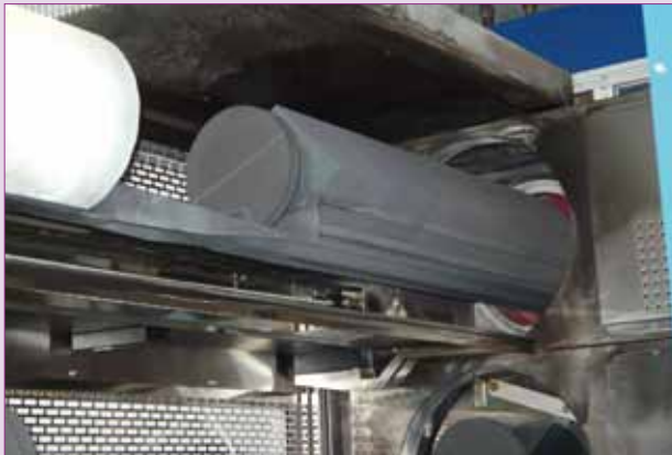
Figure 8. A quartz bot being loaded into a diffusion furnace (SEMCO).
