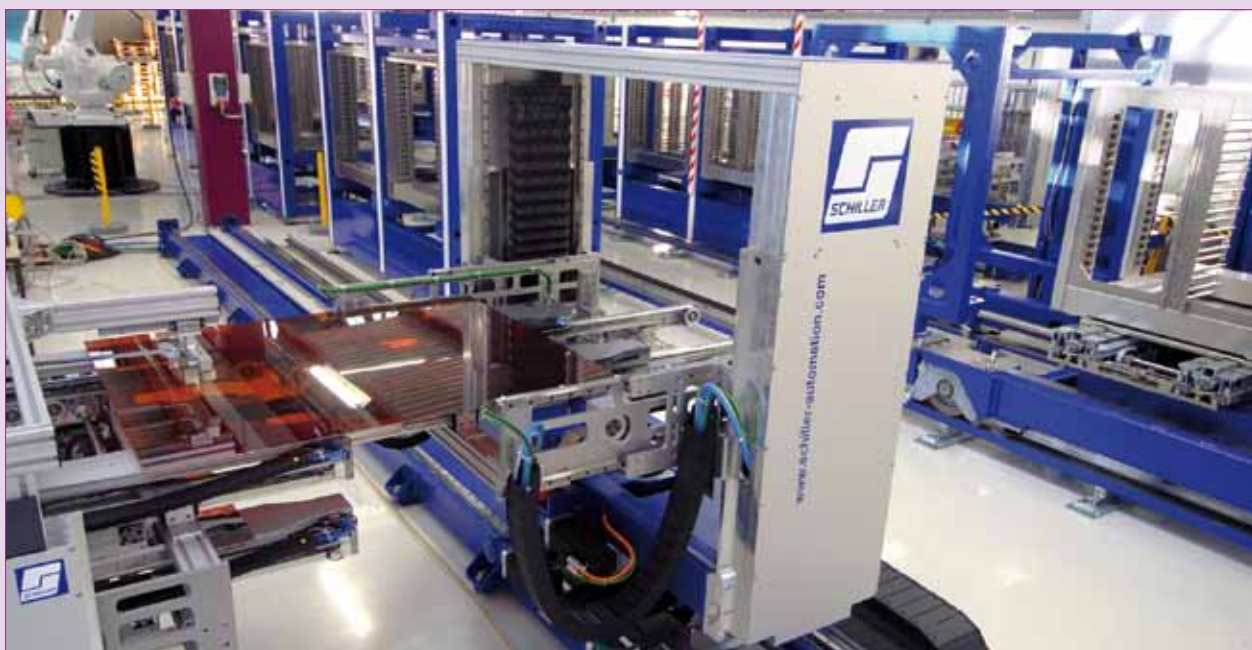
Figure 13. Special transfer solution for unloading and loading of process equipment and cassettes (Schiller Automation).
