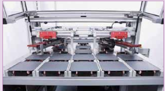
Figure 10. Wafers being dispersed onto several conveyors (AMB).
