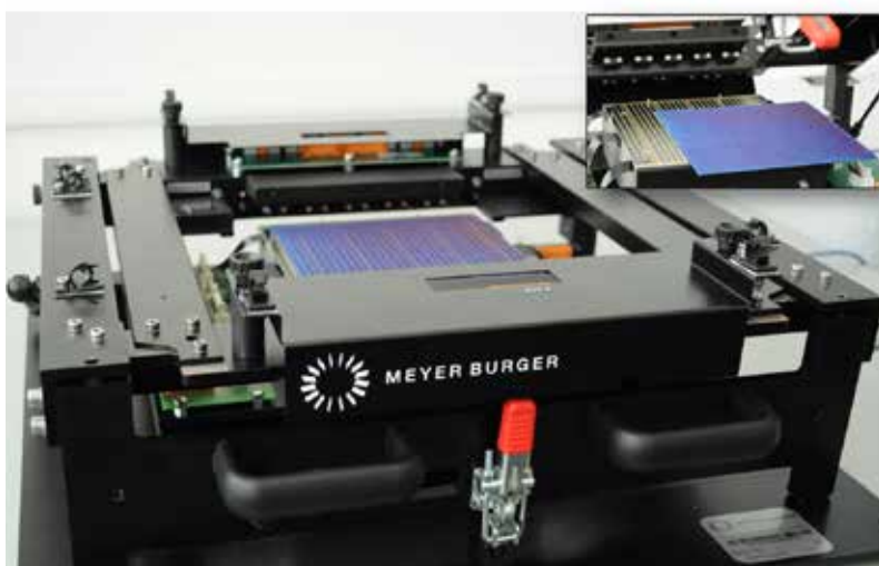
Figure 2. Pasan's bifacial-compatible contacting solution PCB TOUCH , with non-irradiated background and the possibility for background compensation
