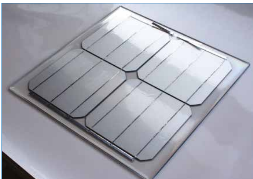
Figure 12. One of the first four-cell mini-modules made from FolMet PERC solar cells (using pre-coated aluminium foil) in combination with standard PV soldering technology.
