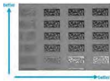
Figure 4. a) Impact on readability through specifying the right process for writing laser marking code; b) impact on readability through specifying the right process for reading laser marking code.
