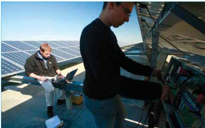
Figure 6. Fraunhofer ISE experts perform field I-V curve measurements.
