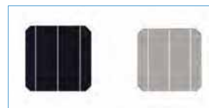
Figure 5. Pictures of the front and back of a production cell fabricated from a 156mm pseudosquare Cz wafer.
