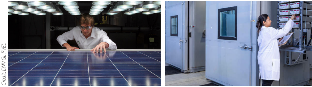
Figure 6. PV module inspection and PV Inverter testing
