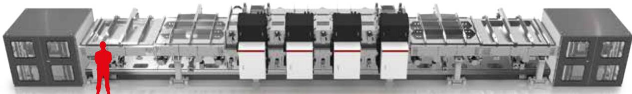
**XEA|nova** horizontal single- & double-sided coating on wafers
