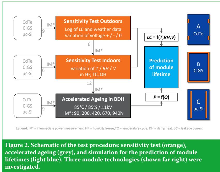
**Figure 2. Schematic of the test procedure: sensitivity test (orange), accelerated ageing (grey), and simulation for the prediction of module lifetimes (light blue). Three module technologies (shown far right) were investigated.**
