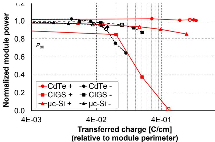
Figure 4. Degradation behaviour of the CdTe, CIGS and  $\mu\text{c-Si}$  modules tested in BDH conditions, as a function of the transferred charge relative to the module perimeter. One set of modules was tested under positive bias (red), the other under negative bias (black). Empty symbols indicate measurements after 420h.
