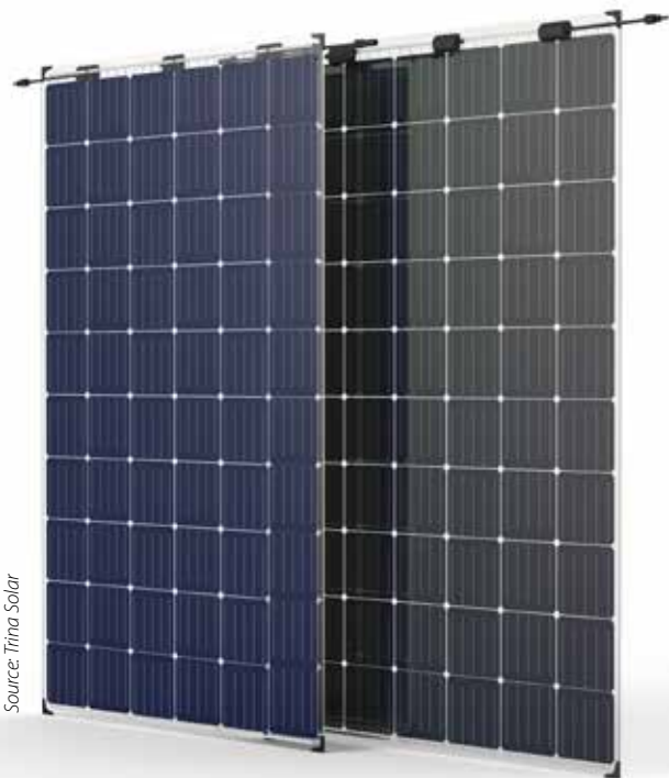
Figure 2. The DUOMAX Twin bifacial module from Trina, featuring a frameless glass/glass configuration with 60 monocrystalline cells (5BB) and p-type PERC cell technology; the reported bifaciality factor is greater than 70%. The module incorporates split junction boxes at the edge with three bypass diodes. The standard glass thickness is 2.5mm on both sides. The module efficiency ranges from 17.6 to 18.9% under STC conditions.
