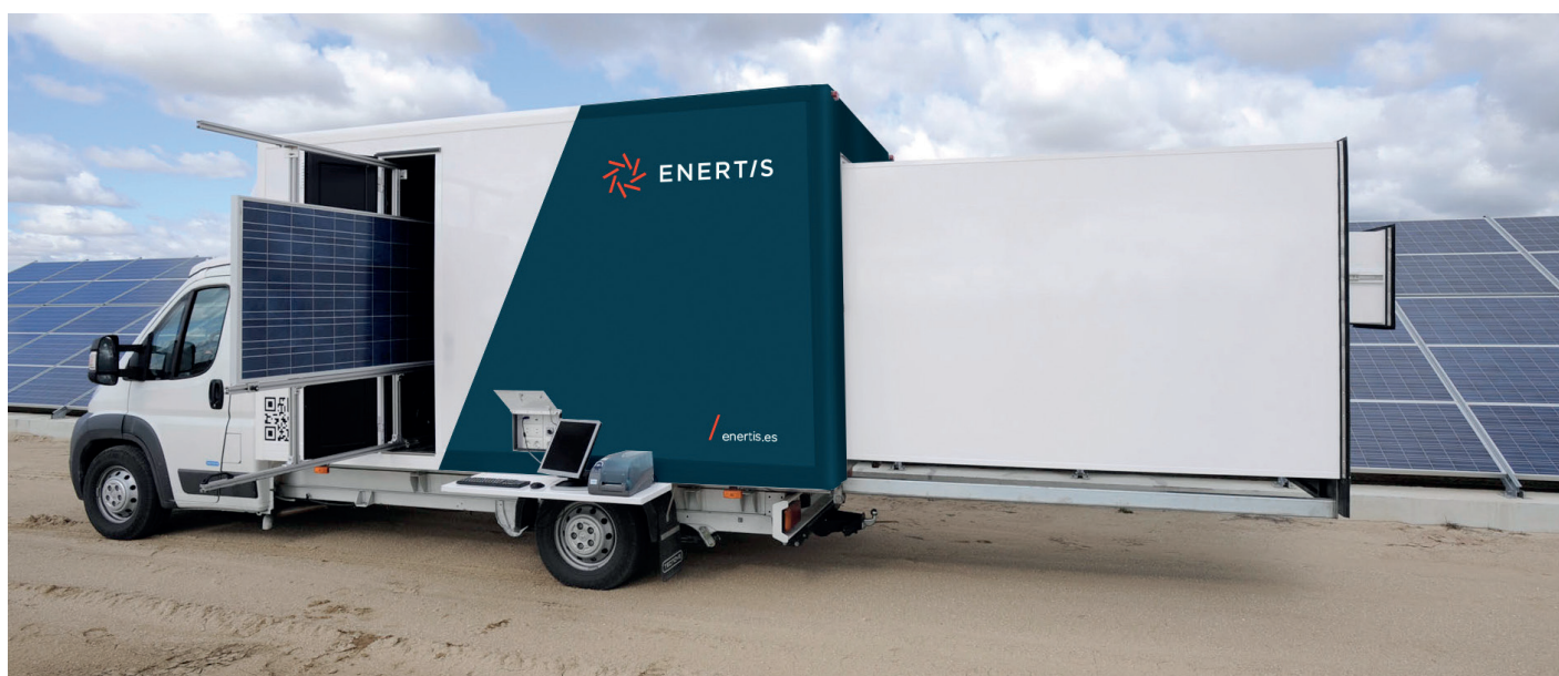
Figure 2. Enertis' PV Mobile Lab.
