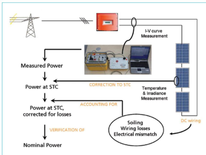
Figure 7. The three steps involved in verifying module power in the field I-V curves.
