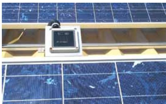
Figure 9. The recalibration value of the majority of recalibrated sensors lies within  $\pm 2\%$ . The measurement uncertainty for cell calibrations is  $\pm 2\%$  at a 95% significance level. Below: A Fraunhofer ISE crystalline silicon reference sensor.
