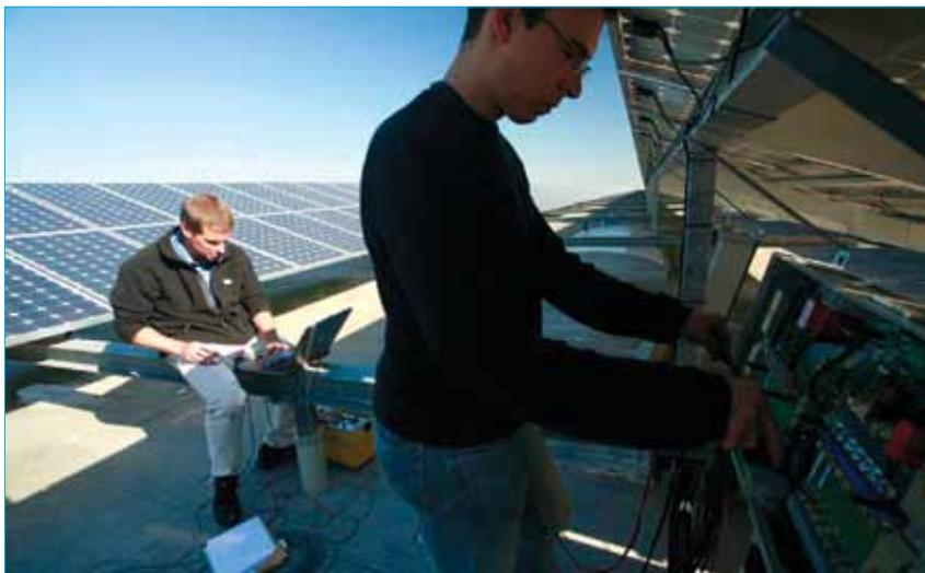
Figure 6. Fraunhofer ISE experts perform field I-V curve measurements.
