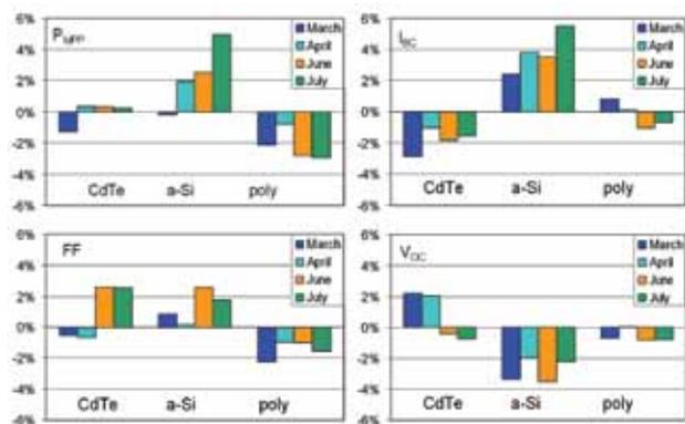
Figure 8. A good agreement of outdoor measurements performed on small PV strings during 2010 with CallLab PV Modules' measurements confirms the accuracy of thoroughly performed field measurements.
