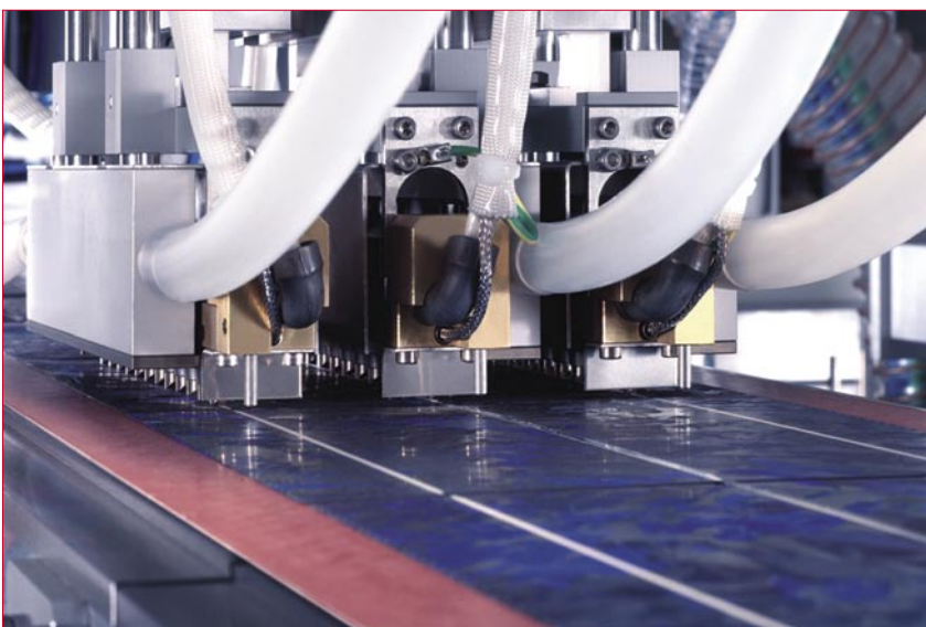
Figure 6. SOMONT’s ‘soft touch’ soldering technology.
