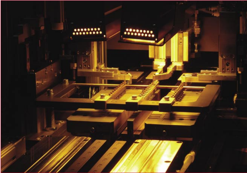
Figure 4. Mondragon preheating station, soldering station and cell holding elements.
