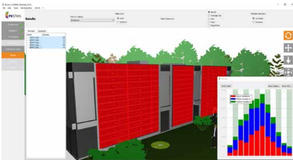
Figure 7. Visualisation of a BIPV project with the PVSITES software tool (CADCAMation). The user is guided through the different project steps, from the computation of solar irradiance on all model surfaces to the system's economic assessment
