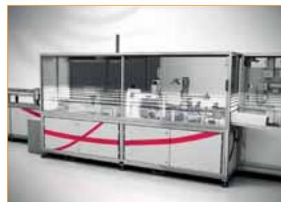
**Mondragon Assembly has developed a high-throughput 150MW 'Front Line' tabbing and stringing system**
