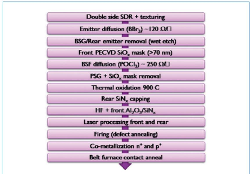
Figure 4. Outline of the nPERT+ cell process sequence.
