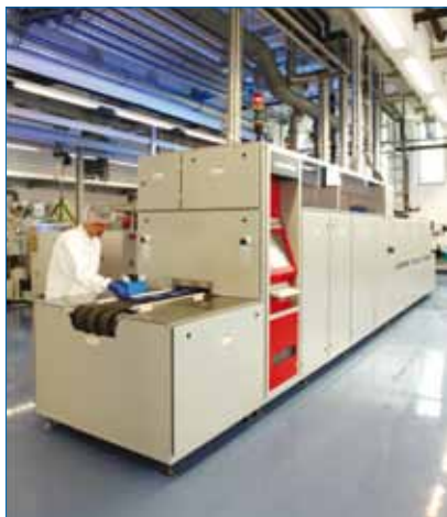
Figure 6. Contact formation of screen-printed solar cells in a conveyor-belt furnace at ISFH.
