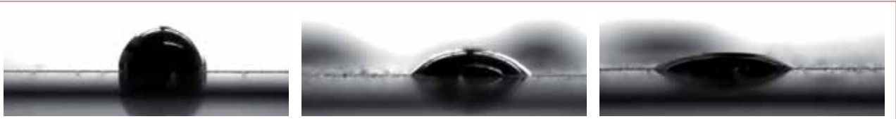
Figure 12. Wetting angle measurement for molten solder balls on cell busbar.
