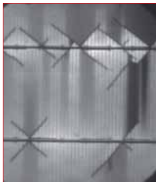
Figure 16. EL image of cell with heavy soldering-induced cracks.
