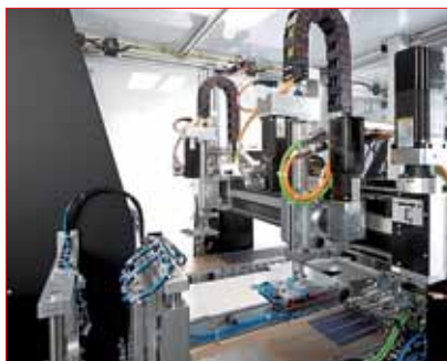
Figure 7. Vision system for initial cell alignment and control.
