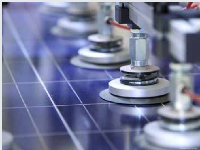
JA Solar modules undergoing a 500 hour PID test.
