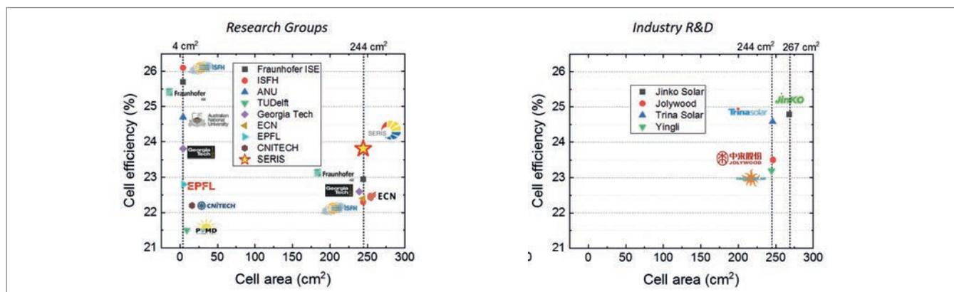
Figure 1. Overview of solar efficiencies achieved with single-side poly-Si/SiO<sub>x</sub> passivating contact stacks on small-area (<100cm<sup>2</sup>) and large-area ( $\geq 239\text{cm}^2$ ) silicon wafer solar cells for various groups and industrial players, as reported at scientific conferences and in the press.
