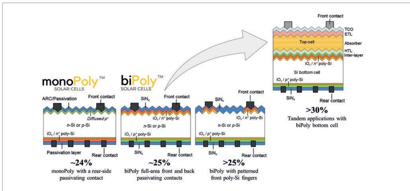
Figure 6. Schematic roadmap depicting the evolution of current PERC cell technology to monoPoly, biPoly and biPoly<sup>+</sup> as the bottom cell in silicon-based tandem solar cell applications.
