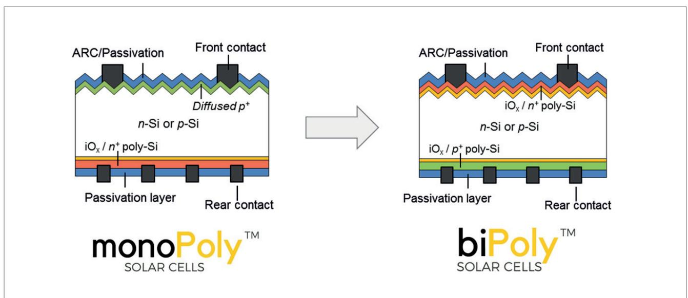
Figure 2. Transition from a bifacial monoPoly cell to a bifacial biPoly cell with a front semitransparent electron-selective passivating contact stack and a rear hole-selective passivating contact stack.
