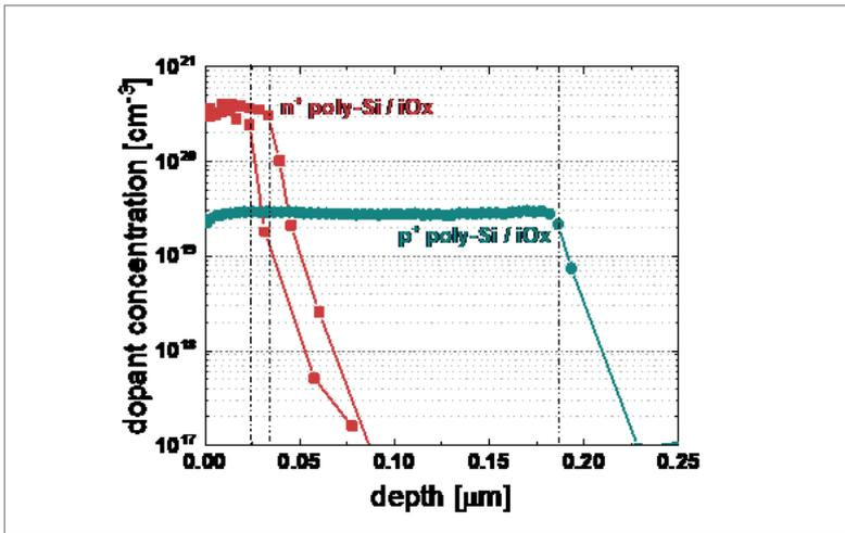
Figure 3. Dopant profiles for ultrathin n<sup>+</sup> poly-Si (25 and 35nm) and p<sup>+</sup> poly-Si (180nm) on iO<sub>x</sub> stacks developed for the biPoly cell structure.
