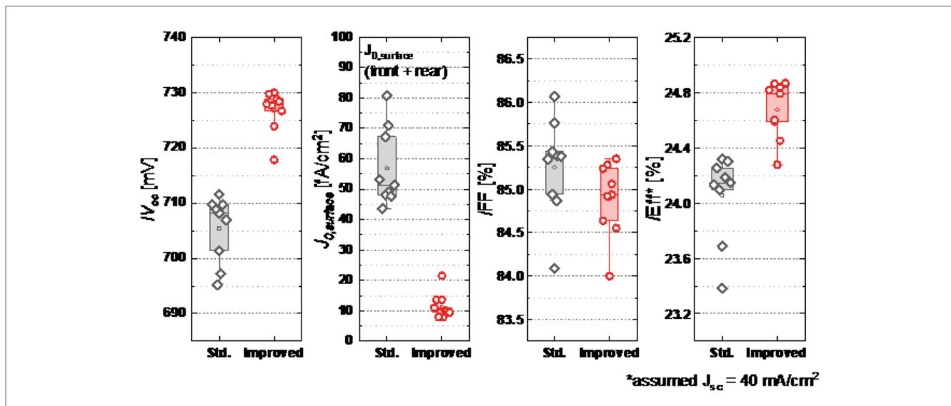
Figure 5. Implied open-circuit voltage ( $iV_{oc}$ ) at 1 sun, total surface recombination current density ( $J_{0,surface}$ ), implied fill factor ( $iFF$ ) and implied efficiency ( $iEff$ ) of biPoly cell precursors fabricated at SERIS. Parameters are measured prior to metallization for standard and optimized process flows. A  $J_{sc}$  of  $40\text{mA}/\text{cm}^2$  is assumed for  $iEff$  estimations.
