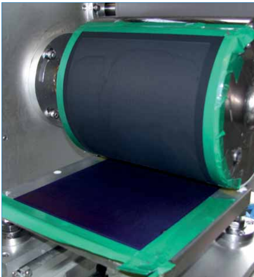
Figure 10. Nissha Angstromer S15 flexographic printing machine with a ContiTech Laserline fine-line printing plate and a Cz-Si precursor fixed on the vacuum table.
