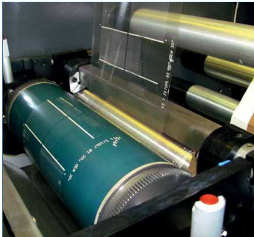
Figure 3. The RSP unit of the Gallus EM 280 label printing machine, which was used for the experiments. This printing machine allows a printing speed of up to v = 100\text{m/min} . (1.7m/s).
