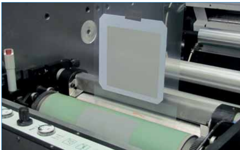
Figure 6. Transport of a Si wafer through the RSP printing unit by fixing it on a foil web.
