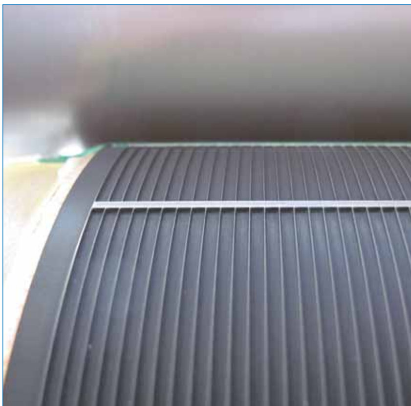
Figure 11. ContiTech Laserline laser-engraved flexographic EPDM printing plate with a fine-line H-pattern layout for seed-layer metallization.
