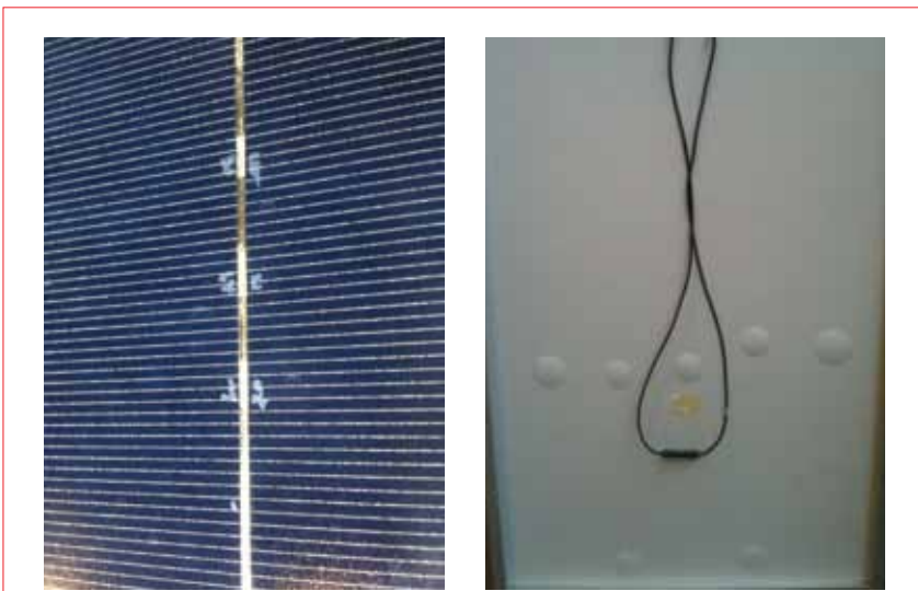
Figure 2. Front-contact-cell modules after a multistress simulator test. Solder flux residue along the interconnect ribbon caused delamination bubbles (left), while lay-up tape outgassing caused backsheet bubbling (right).
