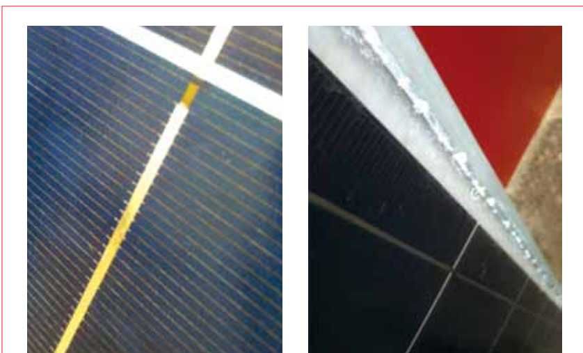
Figure 3. Following 600 hours of damp heat with voltage bias for front-contact-cell modules, corrosion can be seen on the front-contact metal (left). The right-hand picture shows the view looking down the edge of the aluminium frame that surrounds the laminate glass.
