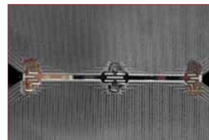
Figure 4. A strain-relieved cell interconnect between two back-contact cells. The three solder bonds on each cell, combined with the plated copper connections between those bonds on the cell, create redundancy.
