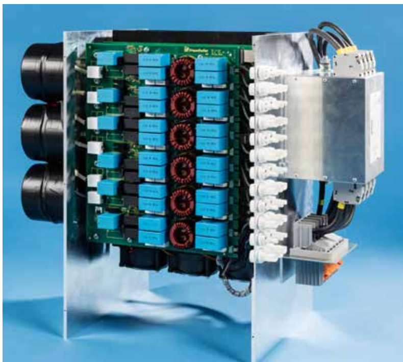
Figure 4. PV-Pack 70kVA PV inverter with new cooling concept
