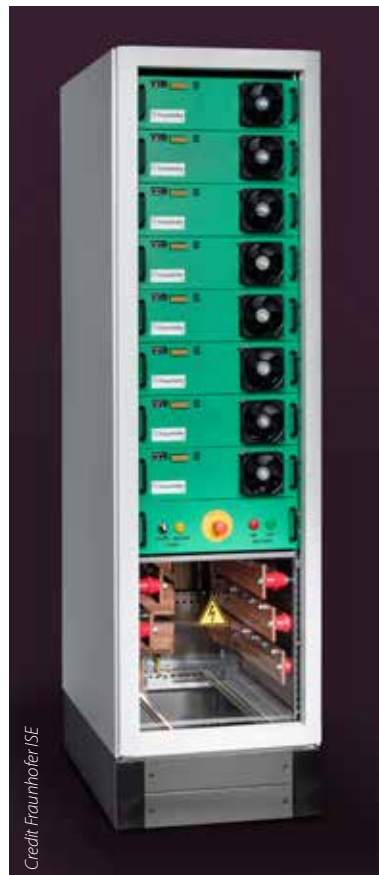
Figure 3. Demonstrator system of a modular, highly compact 1MW battery inverter using SiC-MOSFET's
