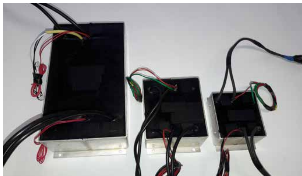
Figure 1. Example of weight/volume reduction of inductors
