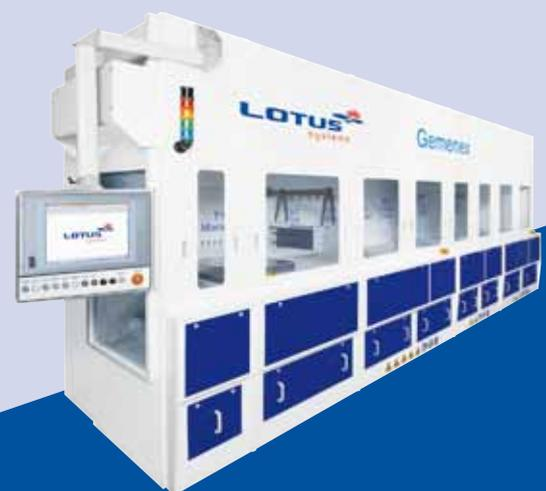
Conceptually, in-line processing should be preferable (with respect to batch processing) as it creates a streamlined production line. In-line processing also offers better 'selective' access to one side or the edges only. In view of the high throughput, measures have to be put in place to swiftly overcome wafer breakage events without noticeable down time.
