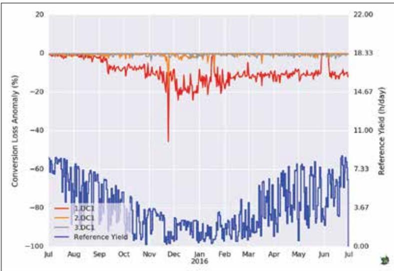
**Figure 5. Conversion loss anomaly for current-based array losses per day, comparing the conversion losses of all arrays/inverters to the best in class of each day. The blue line shows the reference yield and hence the available irradiation for each day. Starting on 11 September 2015, the losses for inverter 1 (red) are much higher than for the others**
