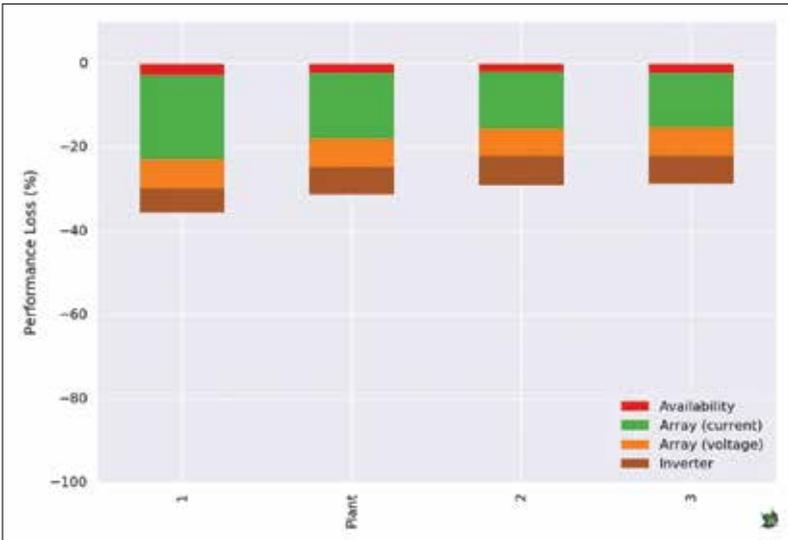
**Figure 4. Performance losses split into loss types and stacked for each array/inverter and the entire plant, sorted in ascending order; particularly the current-based losses (green) are generally too high and worst of all for array/inverter 1; the losses are normalised to the reference yield. Data from 1 July 2015 to 30 June 2016**
