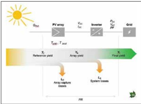
**Figure 2: Energy flow in a grid-connected PV system; with measurements of plane-of-array irradiance (G<sub>POA</sub>), DC voltage and current (V<sub>DC</sub>, I<sub>DC</sub>), AC power, voltage and power factor (P<sub>AC</sub>, V<sub>AC</sub>, PF), ambient and module temperature (T<sub>amb</sub>, T<sub>mod</sub>); yields (Y), losses (L) and performance ratio (PR)**
