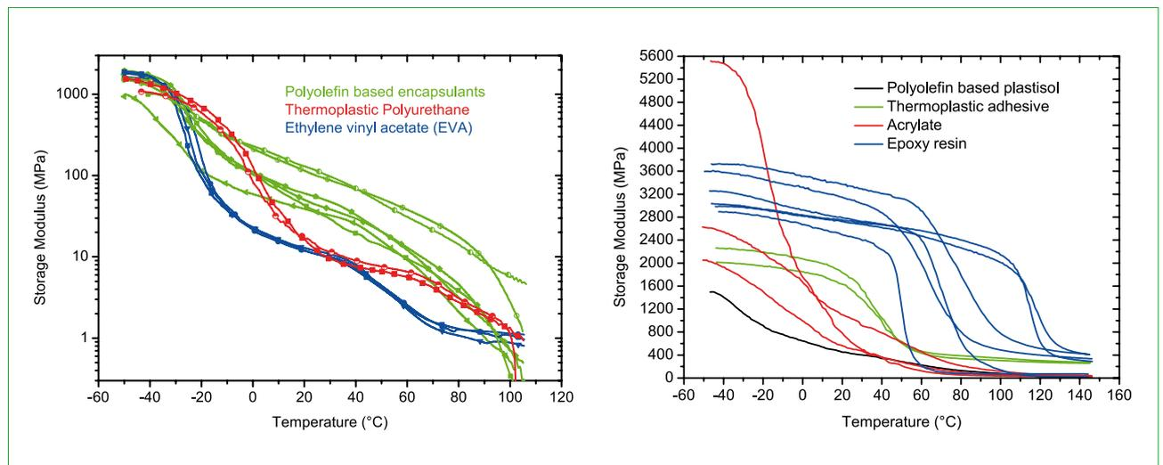
Figure 6. Storage modulus vs. temperature for different encapsulants (left) and polymer conductive adhesives (right).
