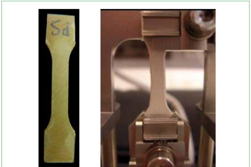
Figure 4. Test specimen made from conductive adhesive (left), and in the testing position (right) for linear DMA.
