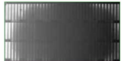
Figure 9. Electroluminescence image of a mini-module showing degradation caused by moisture ingress through the front barrier film.
