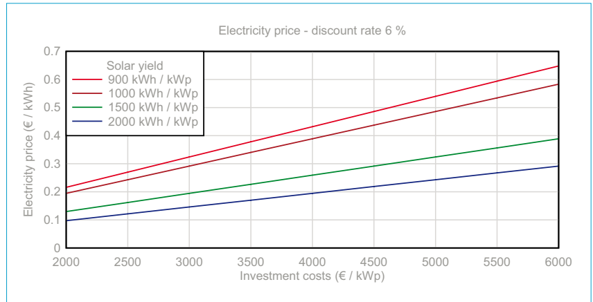
Figure 5. Electricity price for 6% discount rate and 20-year system lifetime for different yield rates.
