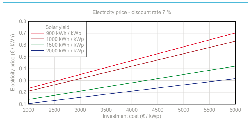
Figure 6. Electricity price for 7% discount rate and 20-year system lifetime for different yield rates.
