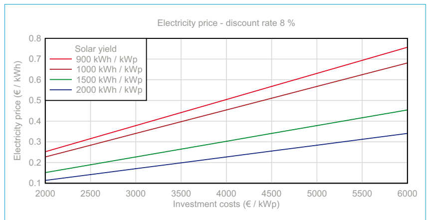
Figure 7. Electricity price for 8% discount rate and 20-year system lifetime for different yield rates.
