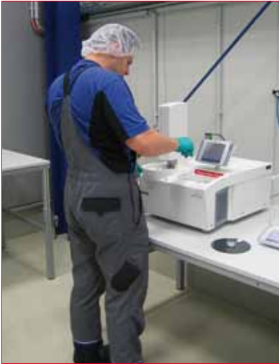
Figure 6. Qualification of uncured EVA film as part of the inspection of incoming goods.
