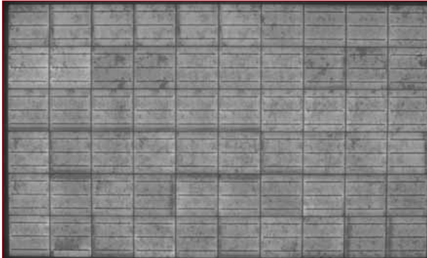
Figure 2. Electroluminescence image of a solar module.
