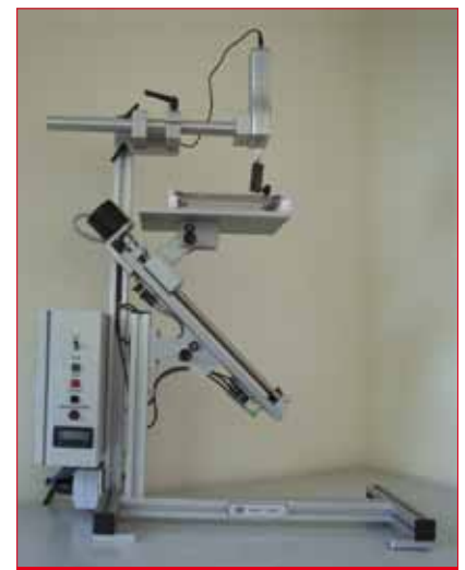
Figure 4. Device for performing a pull-off test on soldered solar cells.
