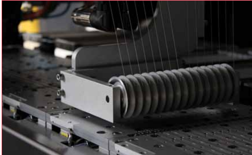
Figure 3. Multi-busbar connector: vacuum chuck used to align the 15 Cu wires on the solar cell.
