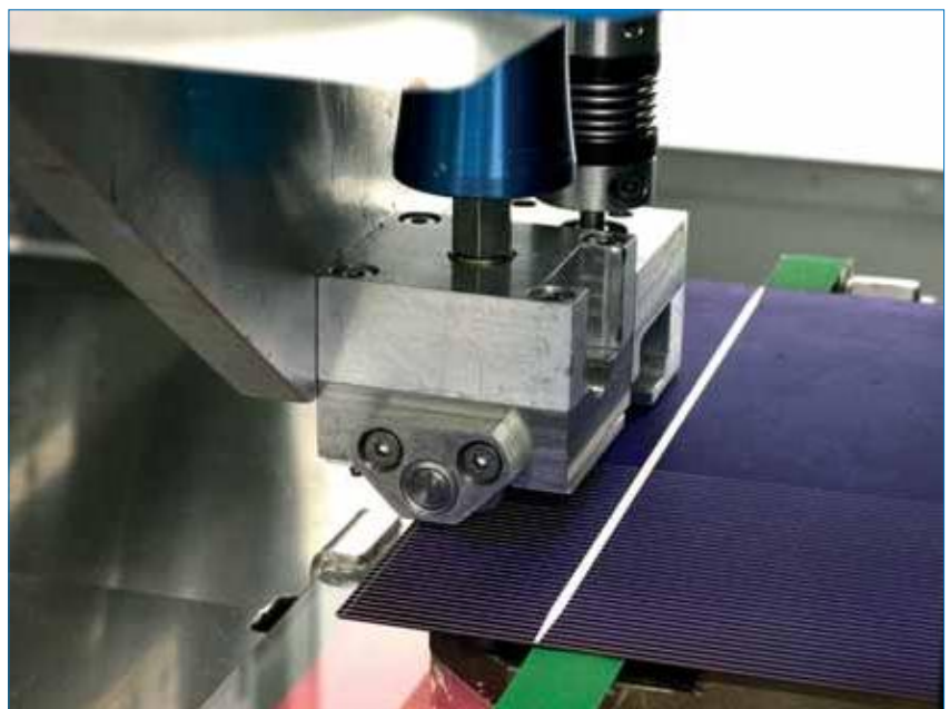
Figure 3. Ten-nozzle print head during solar cell metallization. With this system, process speeds above 600\text{mm}\cdot\text{s}^{-1} can be realized.
