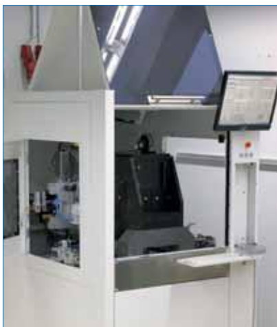
Figure 4. Novel inline-applicable dispensing platform developed by ASYS, to be equipped with multi-nozzle print heads and auxiliaries.
