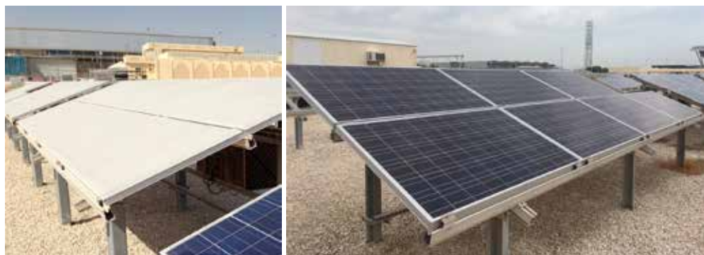
Figure 1. Examples of soiled modules (left) and modules naturally cleaned by heavy rain (right). These are the same test beds viewed from opposite side at the QEERI Outdoor Test Facility
