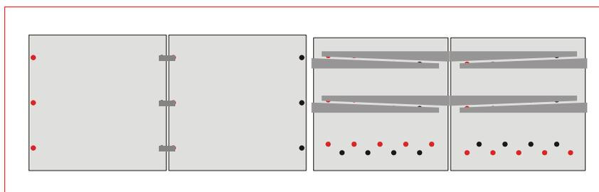
Figure 2. Interconnection schematic for cells with edge contacts (left) and distributed contacts (right).
