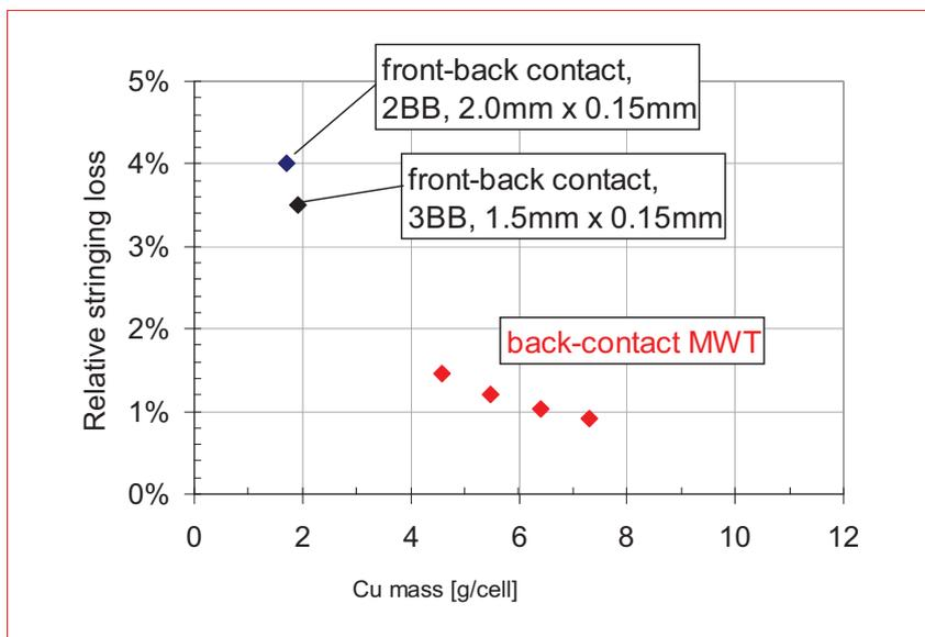
Figure 3. Calculated serial resistance power losses due to cell stringing,  $I_{mpp} = 8.3A$ .
