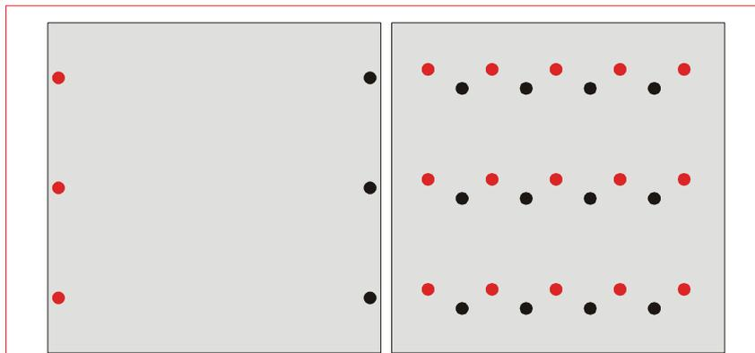
Figure 1. Schematic view of BC cells with edge contacts (left) and distributed contacts (right).
