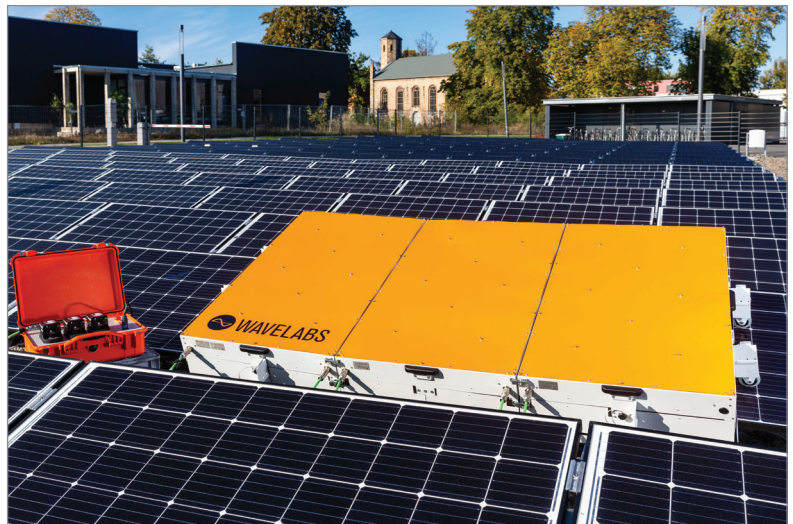
Figure 4. LED-based solar simulator at the Fraunhofer CSP PV park. Using different coloured LEDs, an initial diagnosis of the type of PID can be made.
