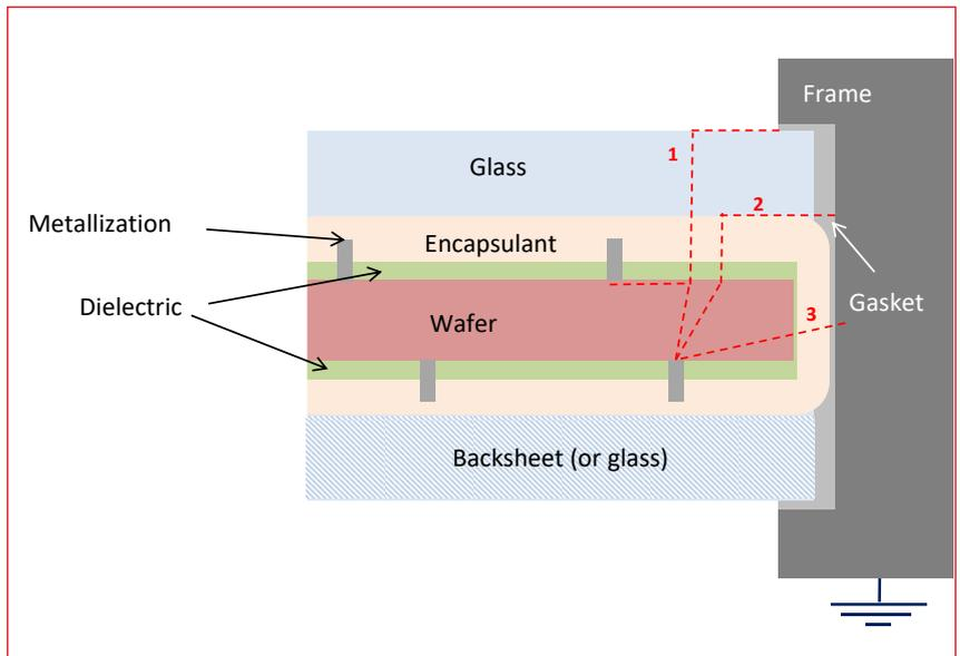
Figure 2. Schematic showing possible leakage current paths (dashed red lines) between the metallization of the cell and the grounded frame (not to scale).
