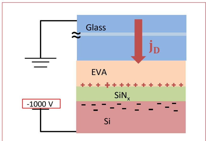
Figure 3. 1D schematic of leakage current at a negative cell bias.
