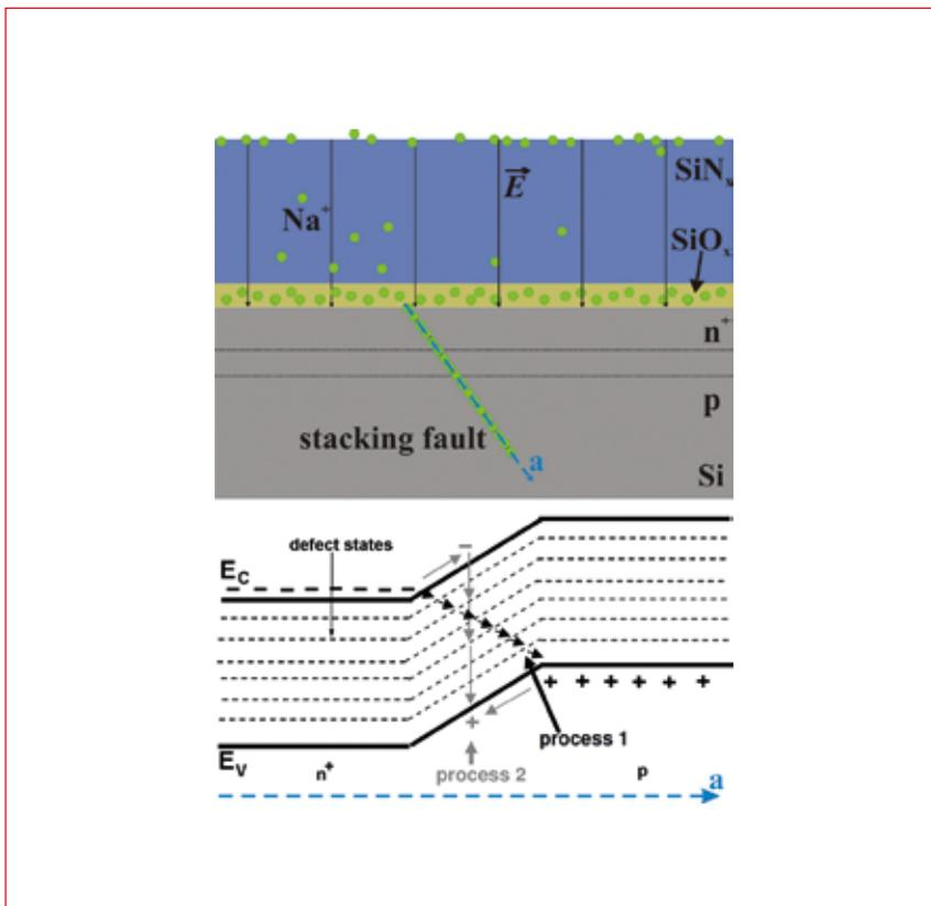
Figure 4. Schematic of a solar cell cross section.  $\text{Na}^+$  ions drift, as a result of the dielectric field, towards the Si interface, where diffusion into stacking faults takes place. The bottom graph shows the proposed band structure along a decorated stacking fault. (Reprinted from Naumann et al. [6] with permission from Elsevier.)
