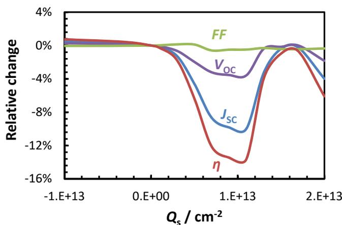
Figure 6. Relative changes in the  $I$ - $V$  characteristics of an n-PERT cell with emitter A.
