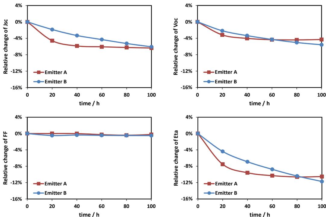
Figure 7. Time evolution of the cell parameters relative to initial values, for n-Pasha single-cell laminates (mini-modules) tested for 100h PID exposure ( $-1000\text{V}$ ,  $60^\circ\text{C}$ ,  $85\% \text{RH}$ ), with a uniform  $n = 1.97 \text{ SiN}_x$  layer on emitters A and B.
