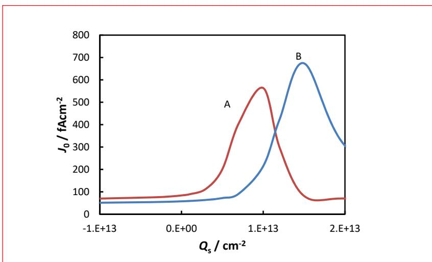
Figure 5. Calculated  $J_0$  values of emitters A and emitter B as a function of an applied external charge  $Q_s$ . The recombination velocity  $S$  at the surface, for holes and electrons, was set to  $2000\text{cm}\cdot\text{s}^{-1}$
