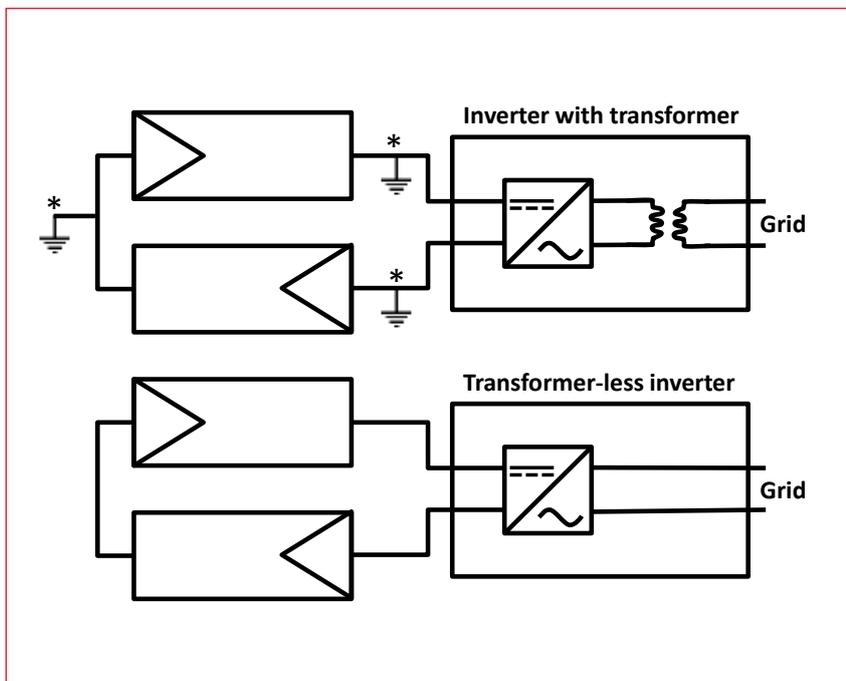
**Figure 1. Schematic of a PV system incorporating an inverter with a transformer (top) and a transformer-less inverter (bottom). The locations indicated with an asterisk and a grounding symbol can be selected (one per circuit) for grounding the circuit of the PV system.**
