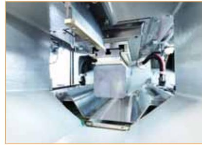
**Meyer Burger's DW288 Series 3 diamond wire cutting tool produces wafers of 145  $\mu\text{m}$  thickness**
