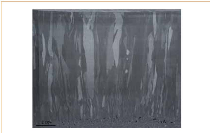
**Figure 5. Photograph of the cross section of a crystallized G1 ingot with a typical HP mc-Si structure. The unmolten feedstock can be seen at the bottom of the ingot.**
