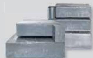
Solar Grade Silicon Ingots from SCU Production System
