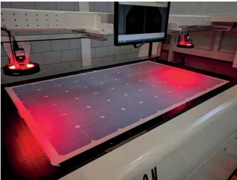
Figure 9: the pick and place stage for the cells on the foil. Picture taken at Eurolab BV, NL.
