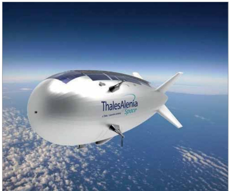
Figure 3. Artist's impression of STRATOBUS, the solar-powered high-altitude pseudo-satellite (HAPS) under development by Thales Alenia Space, with industrialization foreseen in 2020.
