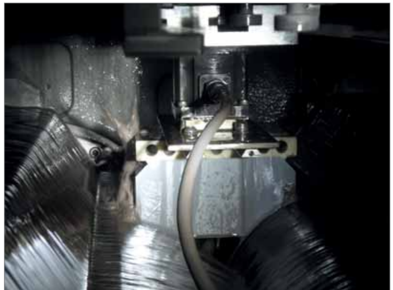
Figure 8. In situ force measurement set-up.
