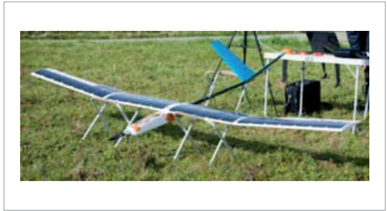
Figure 2. A solar-powered drone co-developed by CEA-INES, commercialized by SUNBIRDS in 2017. The PV module weighs 640g/m 2 .
