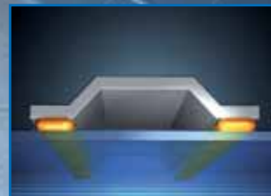
Bonding of back rails
