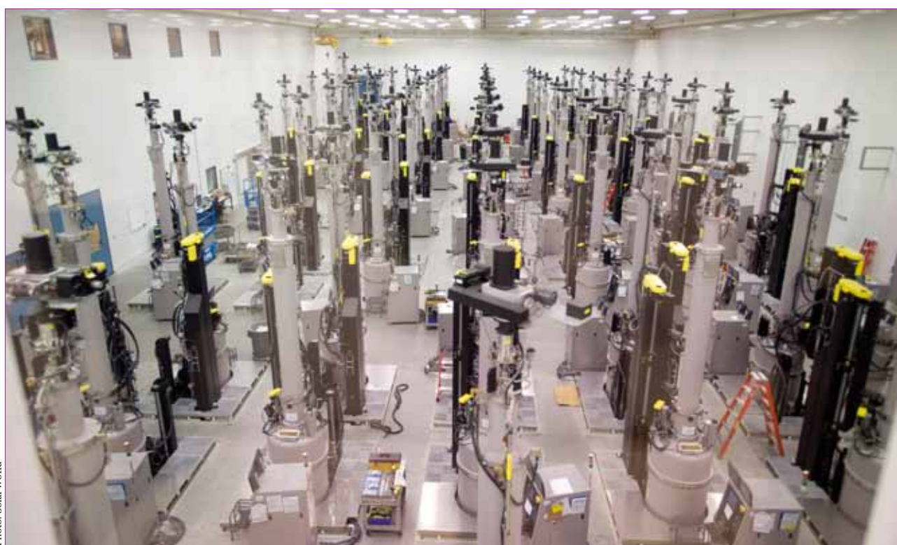
A forest of crystal growers melt down the polysilicon and turn it into ingots.
