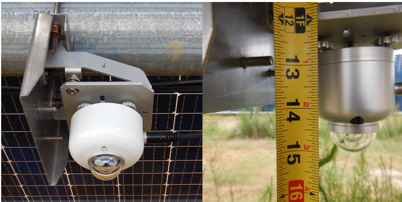
Figure 4. Rear-side pyranometer mount. Options for rear-side pyranometer mounting systems are currently limited and non-standard. Most mounting systems will result in the pyranometer being some distance away from the back of the modules
