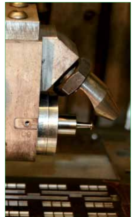
Figure 5. A Sono-Tek spray deposition nozzle. This nozzle is part of a research deposition system at NREL.
