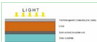
Figure 1. CIGS module cross section.
