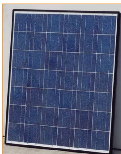
Figure 11. The appearance of the practical-sized module (1165mm × 990mm) made up of 42 screen-printed CDS solar cells.
