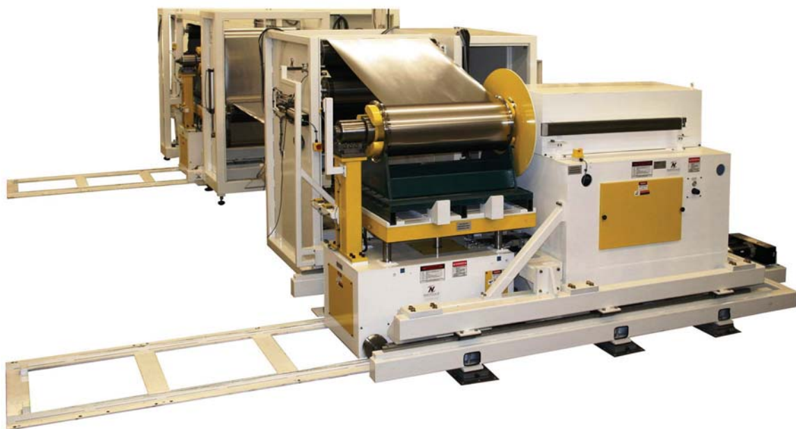
Figure 4. A 12,000lb (5455kg) heavy roll system developed for flexible thin-film PV applications by Northfield Automation.
