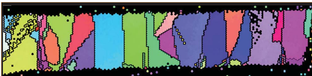
Figure 8. Cross-sectional map of crystalline orientations (black: blank). CDS Si wafers had a quite small grain size, but contained columnar grain structures and good grain boundaries, elements that are suitable for solar cells.
