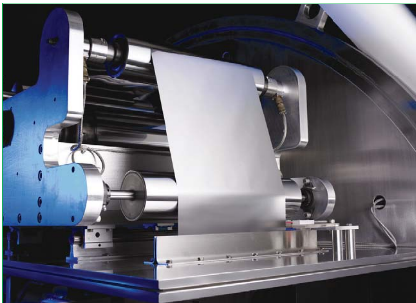
Figure 2. The web payout system of the molybdenum and TCO modules on Veeco's FastFlex CIGS processing platform.
