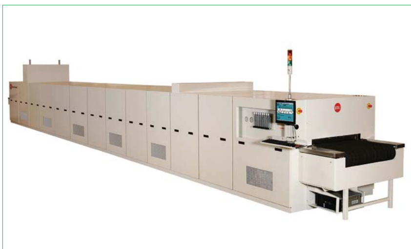
Figure 3. BTU's thin-film PV furnaces offer tight thermal uniformities for CdTe and CIGS manufacturing.
