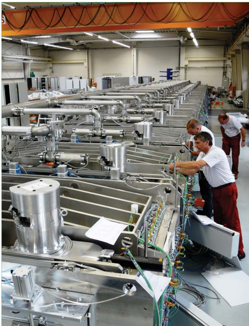
Figure 1. Zinc oxide TCO sputtering tools for CIGS thin-film PV being assembled at centrotherm's factory.
