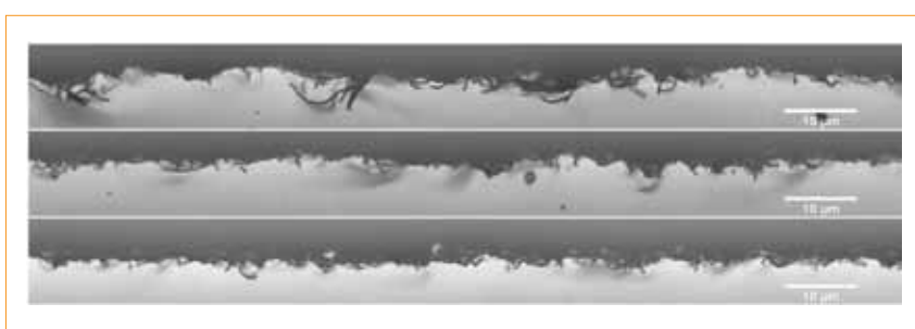
Figure 14. Cleavage edge as observed with a confocal microscope at the wire inlet (top), at the centre of the wafer (middle) and the wire outlet (bottom). Image scope is 120µm × 12µm.
