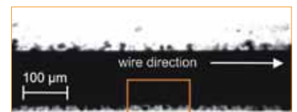
Figure 5. Image of the sawing channel in a glass sample as viewed from the side. The channel is illuminated from the back side with a halogen lamp. The particle movement was observed with a high-speed camera [2].
