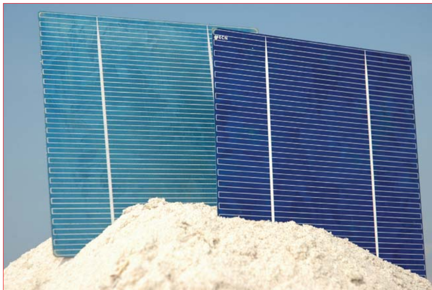
Figure 2. Picture of a open rear-side solar cell. The rear-side is shown on the left and the front side on the right.
