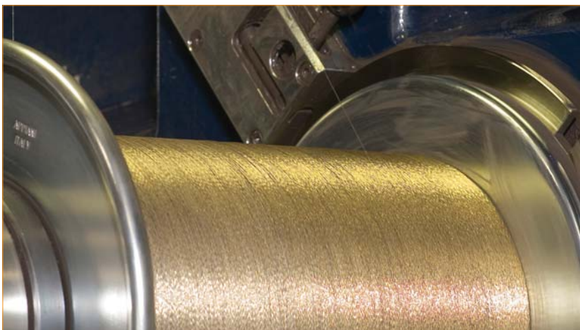
PV Crystalox's ingot cutting wire saw.
