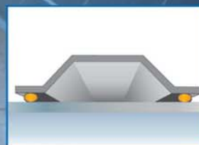
Bonding of back rails
