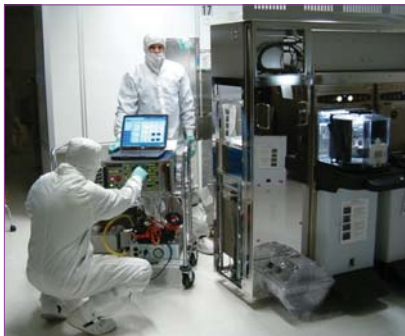
Figure 5. Engineers use an Industrial Power Corruptor (centre) to create calibrated voltage sags. Using these sags and the SEMI F47 standard, specialists from the Power Standards Lab can increase the immunity of almost any equipment to voltage sags, increasing yields and reliability.
