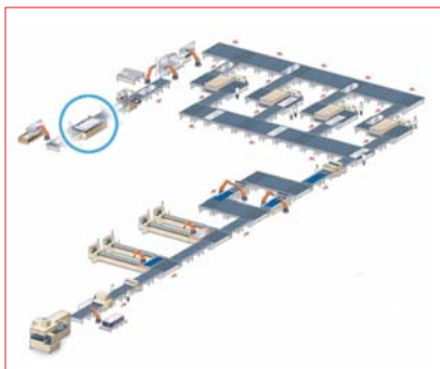
Location of Spire's Solar Simulator on the Spi-Line module production line.
