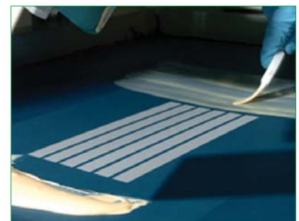
Pasting process in the production of Dyesol's dye solar cell (DSC) technology.
