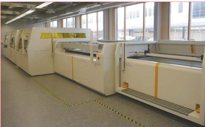
Figure 7. Picture of the pilot line at ECN for manufacturing back-contact modules.
