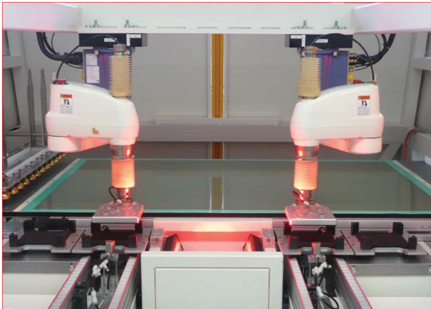
Figure 8. Close-up view of the pick-and-place robots.
