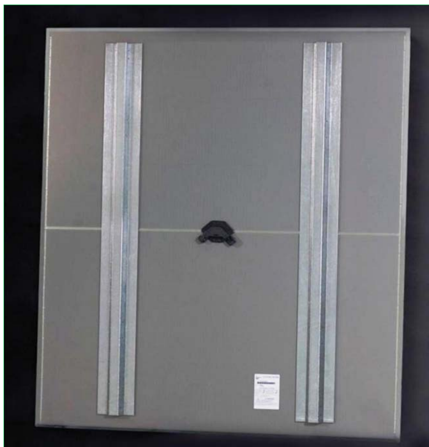
Figure 3. Back-side view of the quarter-size MBTF100 module with bonded back rail.
