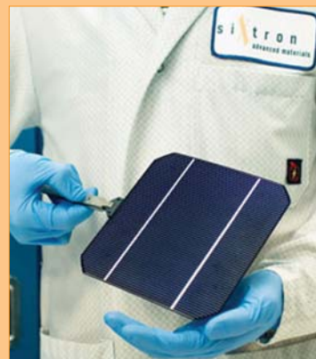
SiXtron's Silexium silane-free antireflective passivation film on a solar cell.
