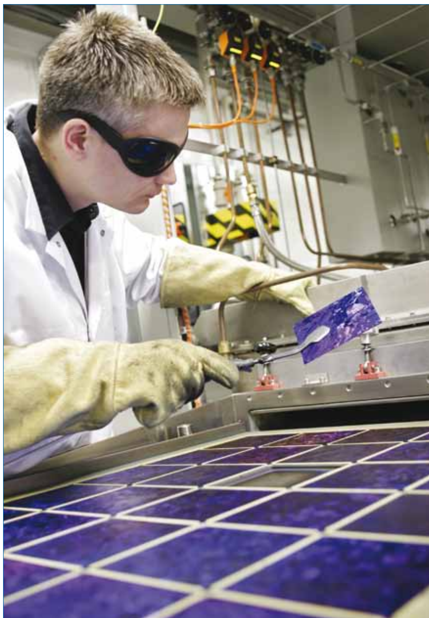
Figure 4. Traditional surface passivation technique: in-line vacuum system for etching, and subsequent passivation by very high frequency PECVD of SiN.
