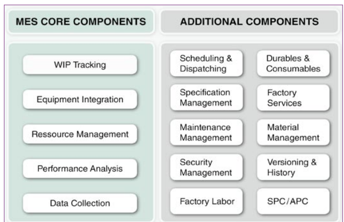
Figure 3. Suggested MES core components for the first stage and additional components that can be integrated in a second step.
